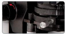
Tighten the thumbscrews to roughly center the substage condenser so that the top lens of the condenser is centered beneath the objective in use. You will more accurately center and focus the condenser when you reach section Koehler Setup.
